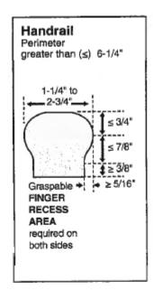
R311.5.6.3 Handrail grip size. All required handrails shall be of one of the following types or provide equivalent graspability.
