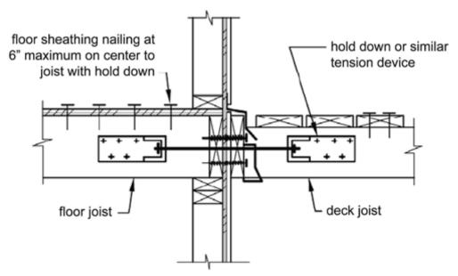
NOTE: An acceptable alternative to the ledger attachment and lateral load tension device requirements is the construction of a free-standing deck with no structural attachment to the house, a professional design may be required.
